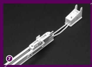
Slide the master carrier underlap, together with the second cord connector into the cord channel of the track and fix the second pulley onto the track. Use the screwdriver.
