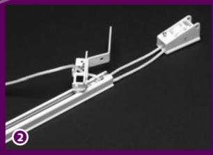
Slide the master carrier, together with the two cord connectors into the cord channel of the track. The cord is lifting out of the track, through the first gap of the master carrier overlap.
