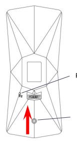
P2 button (for programming tubular motor)
