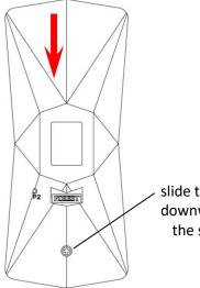
slide the back cover downwards and fix the screw
